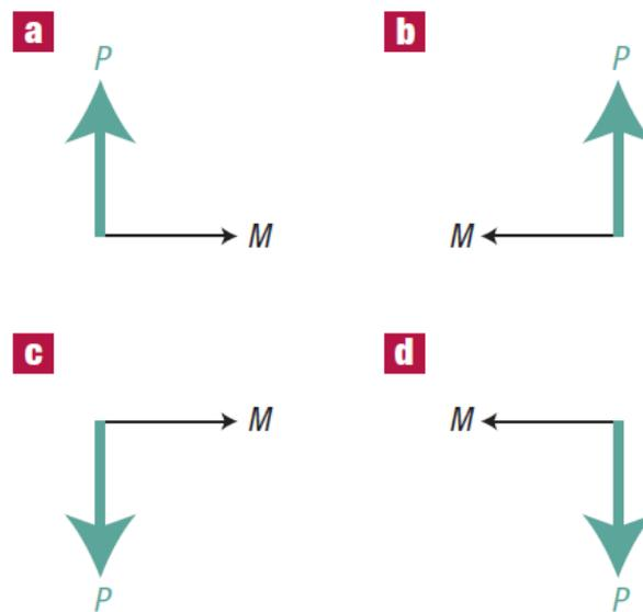
**Figure 1** -The 4 different states possible for the Magnetolectric coupling: (+P,+M), (+P,-M), (-P,+M) and (-P,-M) (ordered from a to d) [4]
