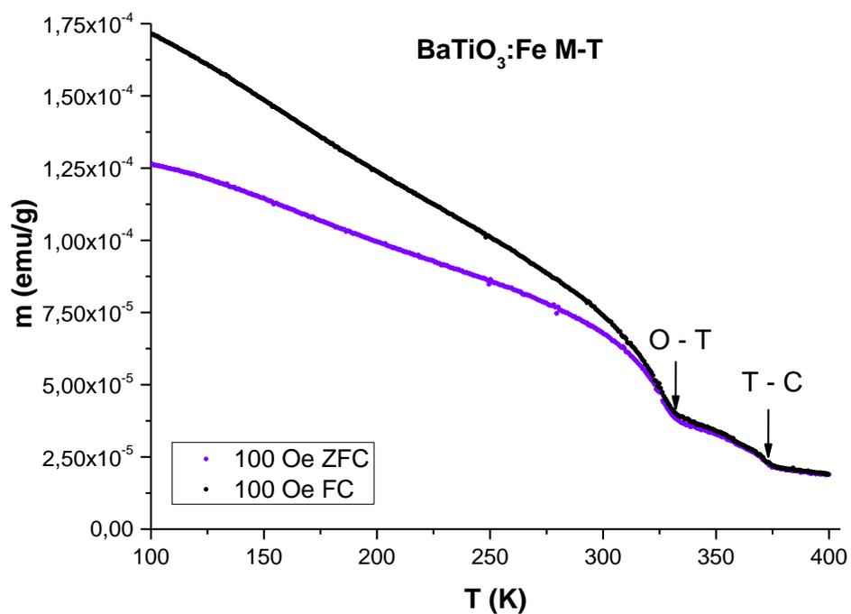
**Figure 2** – Magnetization curve of BaTiO<sub>3</sub>:Fe measured in the IFIMUP SQUID
